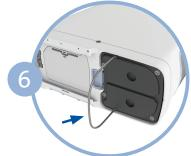
While holding the button open, slide the column assembly out of the device by pulling on the column pull handle.
